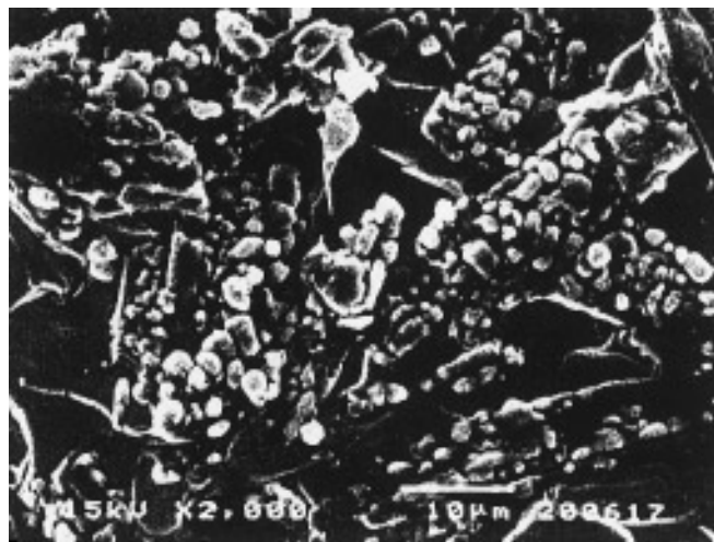
FIG. 11. SEM photograph of decomposed (\text{Bi,Pb}) -2223 phase showing formation of various precipitates.
